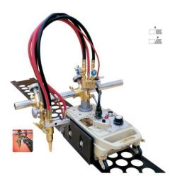
The main body is made of high strength alloy aluminum by die-casting
